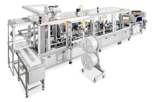
For the production of solution bags in PVC-FREE or NON-PVC film
